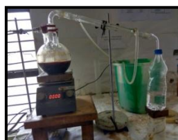
Fig 3: Methanol recovery from distillation process
